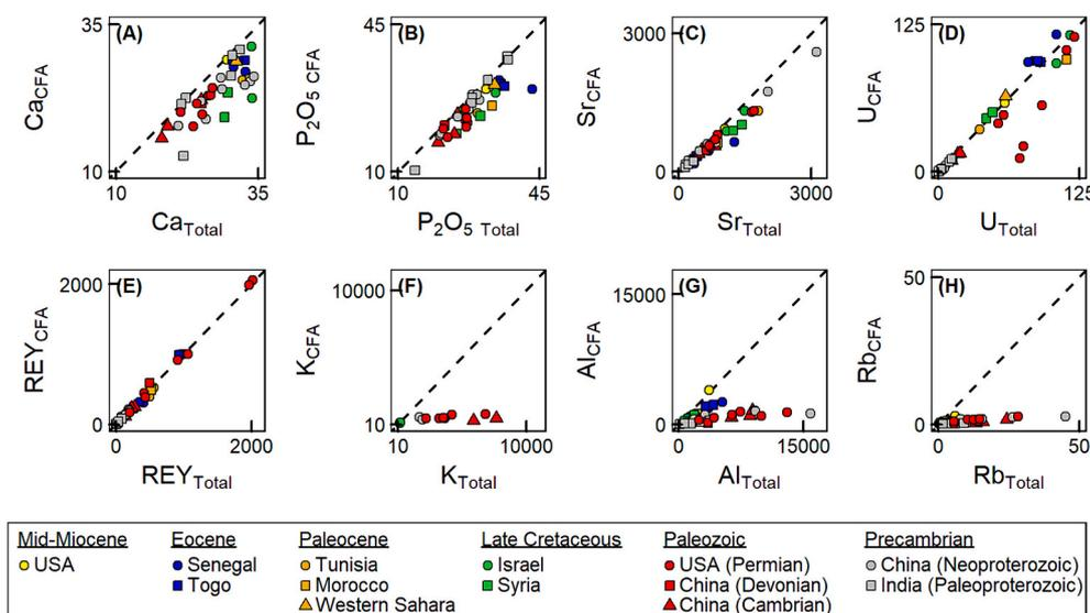
**Fig. 1.** Enrichment of select elements and REY in the phosphate phase (CFA phase) compared to the bulk rock (total digest). Concentration units are mg/kg, with the exception of Ca and P<sub>2</sub>O<sub>5</sub> (wt%). The dashed black line represents a 1:1 concentration ratio between CFA phase and bulk rock. Potassium was not detected above the detection limit for the majority of analyzed CFA phases.
