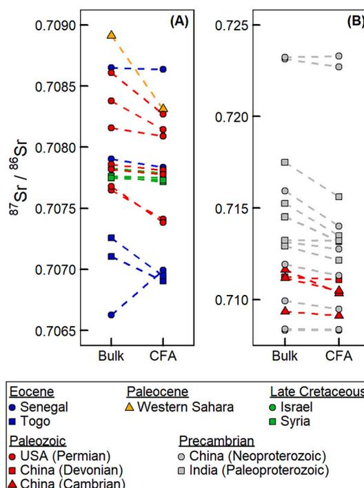
Fig. 6. Comparison of the  $^{87}\text{Sr}/^{86}\text{Sr}$  of bulk phosphate rock (Bulk) and selectively extracted phosphate phase (CFA) conducted through sequential leaching experiments. Data is represented in (A) young and Permian phosphate rocks and (B) old phosphate rocks.
